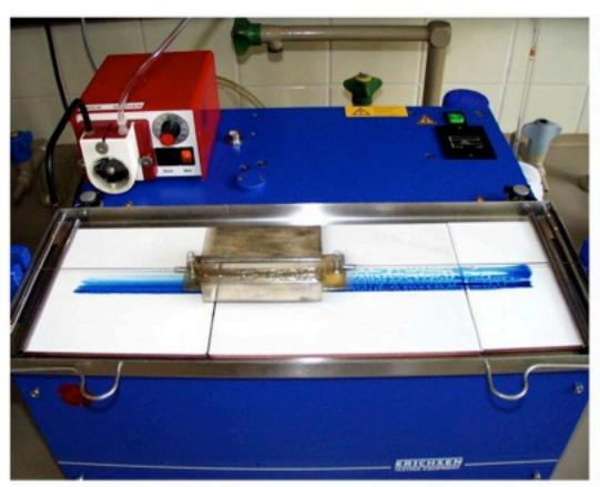
Erichsen Srub Resistance Tester applying abrasive forces with a nylon brush or pads onto the tile surface
